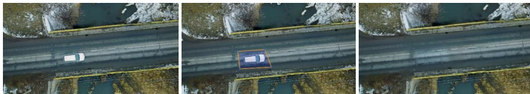
Using the Adjust Stitching Line tool to eliminate moving objects on the street
