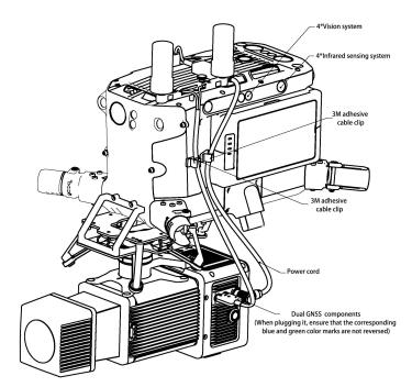
Note: Only when using the RIEGL miniVUX-3UAV, a power cord connection is required.
