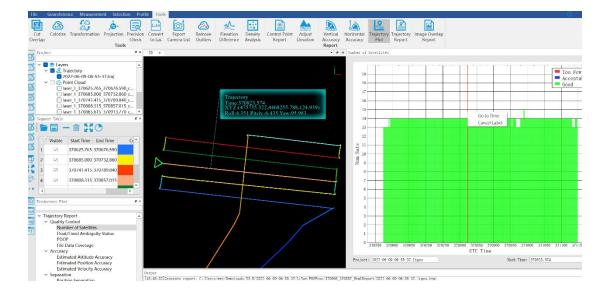
Floating/Fixed ambiguity status: Click to show the plot of ambiguity resolution status. This is used to show the situation of cycle ambiguity resolution. If the status is shown as green on the plot, it means the cycle ambiguity resolution is fixed. If it is red on the plot, it means the cycle ambiguity resolution is floating.
