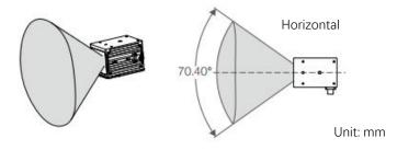
Please note that the effective range of Livox Avia is different in different FOV regions. The closer to the edge of the FOV, the shorter the effective range. Please be careful with the range to avoid incomplete acquisition coverage. The measuring range can refer to the following figure:
