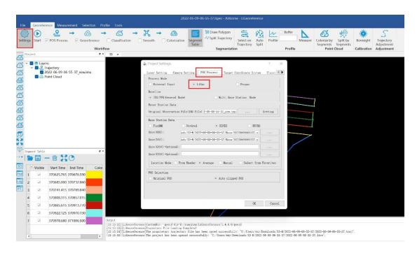
(2) Select the processing mode according to the length of the trajectory. It is recommended to use the general mode. When the length of the trajectory is more than 10 km, the long baseline mode can be selected.
