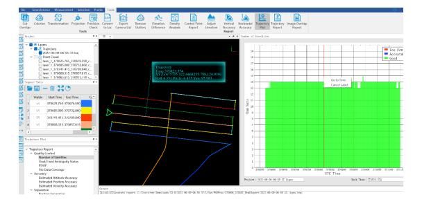
Floating/Fixed ambiguity status: Click to show the plot of ambiguity resolution status. This is used to show the situation of cycle ambiguity resolution. If the status is shown as green on the plot, it means the cycle ambiguity resolution is fixed. If it is red on the plot, it means the cycle ambiguity resolution is floating.
