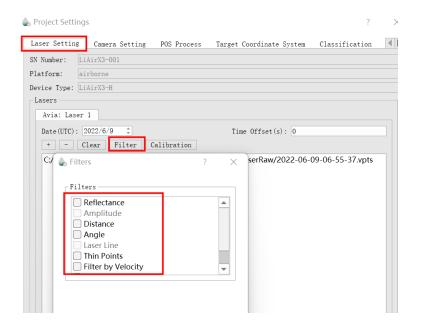
Normally, the user does not need to change the parameters of the laser setting interface. If users want to limit the output power range by reflectivity, distance and scanning angle, users could change the range via clicking "Filter" to set the parameters. For more details, please visit LiGeoreference users guide.
