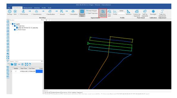
(2) If needed to select multiple trajectories, then repeat the above operation, and the selected trajectory segments will be displayed in the cutting table at the lower left corner.
