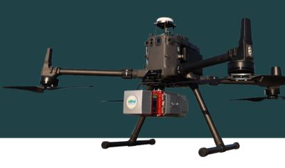
The LiAir 250 Pro system is a lightweight multi-wavelength LiDAR system developed for multi-rotor platforms. It integrates a compact LiDAR system, an inertial navigation system, and a control system to collect massive amounts of high-precision point cloud data and rich image information. It can be used widely in the acquisition of 3D spatial information.
