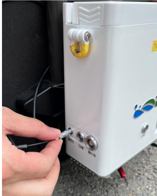
Figure 2-10 The GNSS cable is inserted into the GNSS port of the battery compartment
