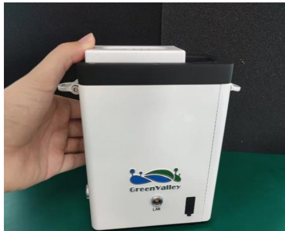
Figure 2-1 Inserting the battery
