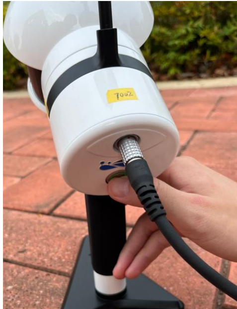
Figure 5-5 Press and hold the button for initialization
