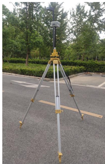
Figure 4-1 Base station erection
