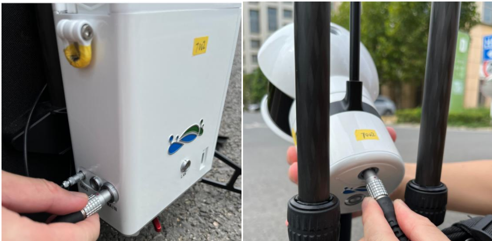
Figure 2-11 Connect the power cable (MAIN port).
