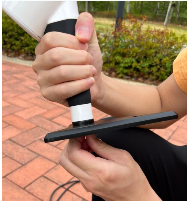
Figure 2-7: Disassembling the dot base
