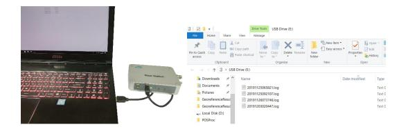
Note: Base station file name in SD card: UTC time + suffix (log), for example: 20170810063808.log.
