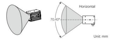
Please note that the effective range of Livox Avia is different in different FOV regions. The closer to the edge of the FOV, the shorter the effective range. Please be careful with the range to avoid incomplete acquisition coverage. The measuring range can refer to the following figure:
