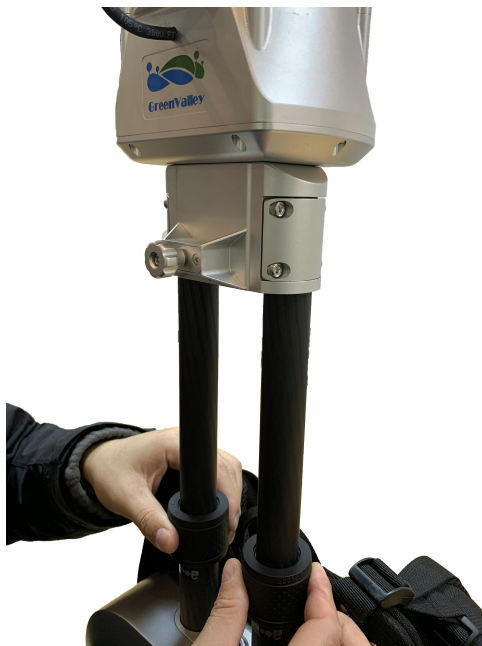
Tighten the lock rings
