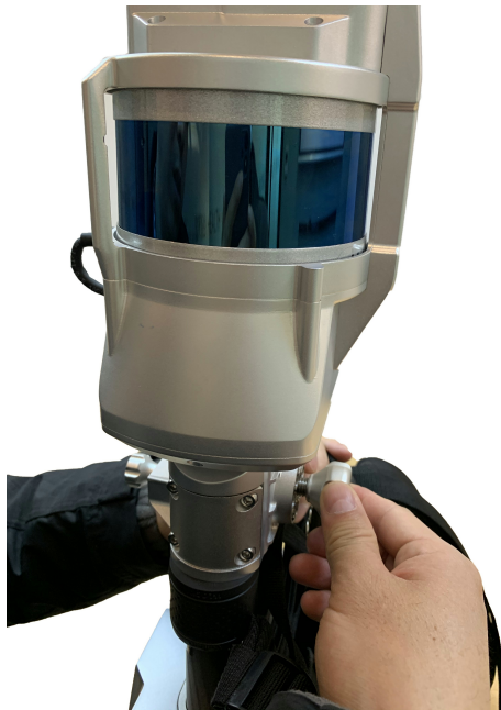
Tighten the screw.
