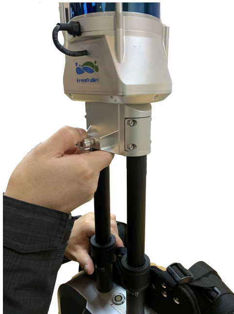
Extend the Scanner Arm
