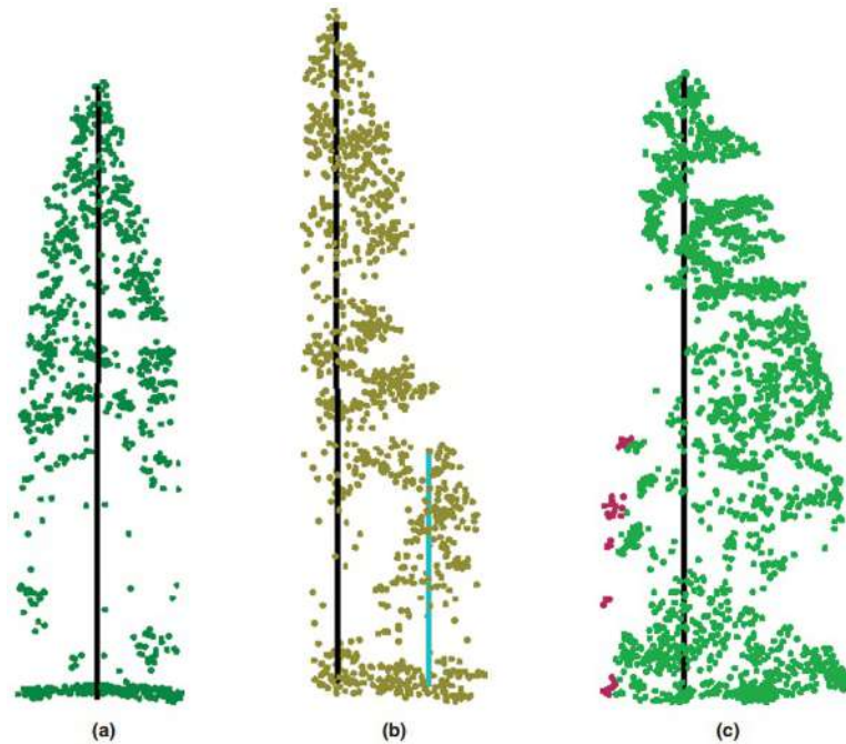
(a) Correctly detected tree (True Positive, TP) (b) undetected tree (False Negative, FN) (c) falsely detected tree (False Positive, FP)
