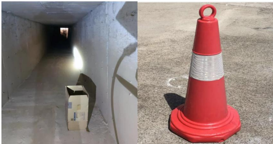
Figure 3-9 Additional feature points for scanning areas such as tunnels/mines
