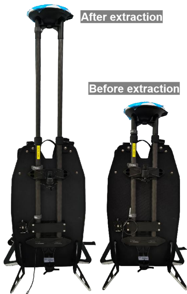
Figure 2-10 Comparison of backpack kit (before and after withdrawal)
