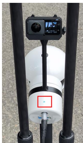
Figure 5-21 Rapid flashing to always-on
