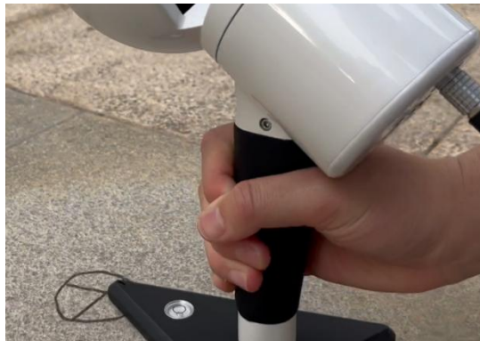
Figure 5-7 GCP collection (Align the "cross" hole with the control point)
