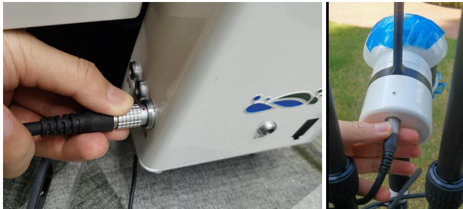
Figure 2-16 Connecting the power cable (MAIN port)
