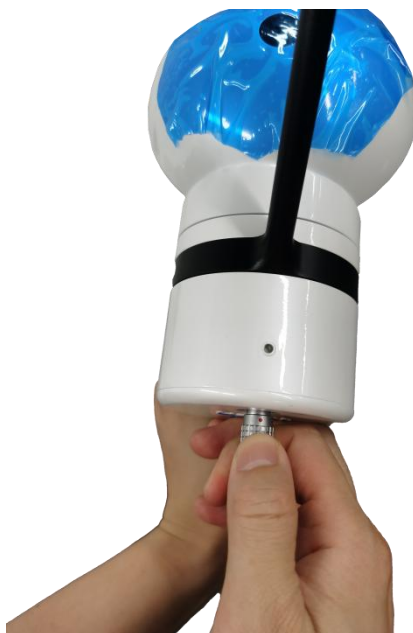
Figure 2-4 Connect the power cord to the host of the handheld device
