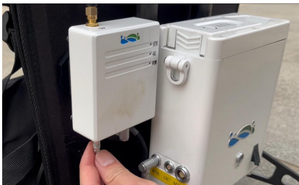
Figure 2-13 Inserting GNSS feeder cable into the GNSS interface of the GNSS module
