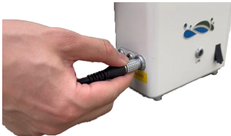
Figure 2-3 Connect the power cable to the battery box (MAIN port)
