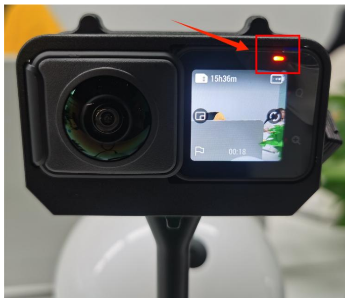
Figure 5-14 Starting recording on the camera automatically
