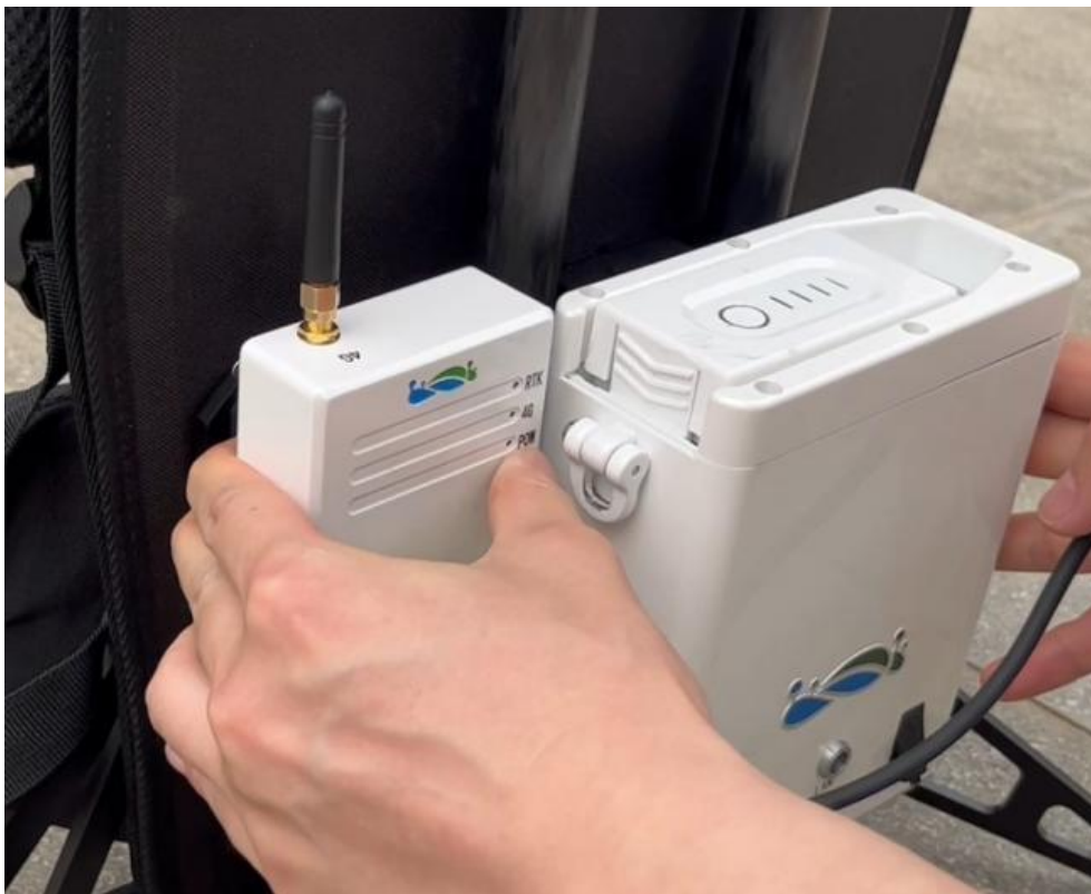
Figure 2-12 Fixing the GNSS module on the kit base
