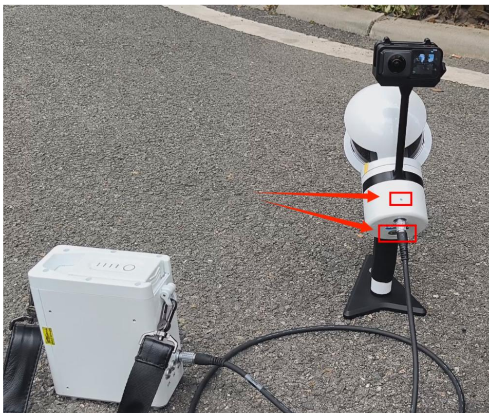
Figure 5-12 Rapid flashing to always-on
