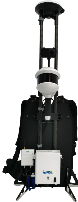
Figure 1-3 LiGrip H120 and backpack kit (For details, see the relevant kit information)
