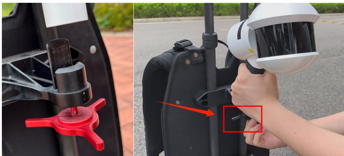
Figure 2-11 Using the hand to hold the bottom to align with the top and insert it and tightening with screws
