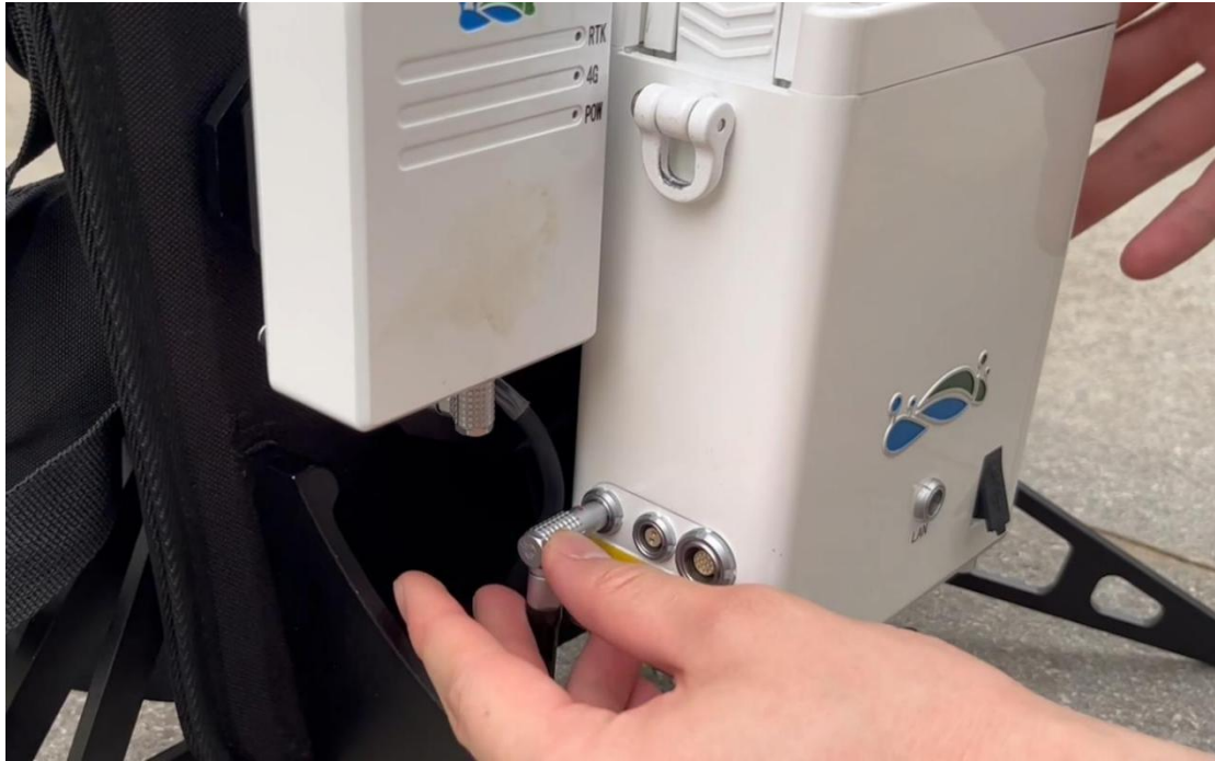
Figure 2-14 Inserting the RTK cable into the RTK interface of the main unit box and GNSS module respectively
