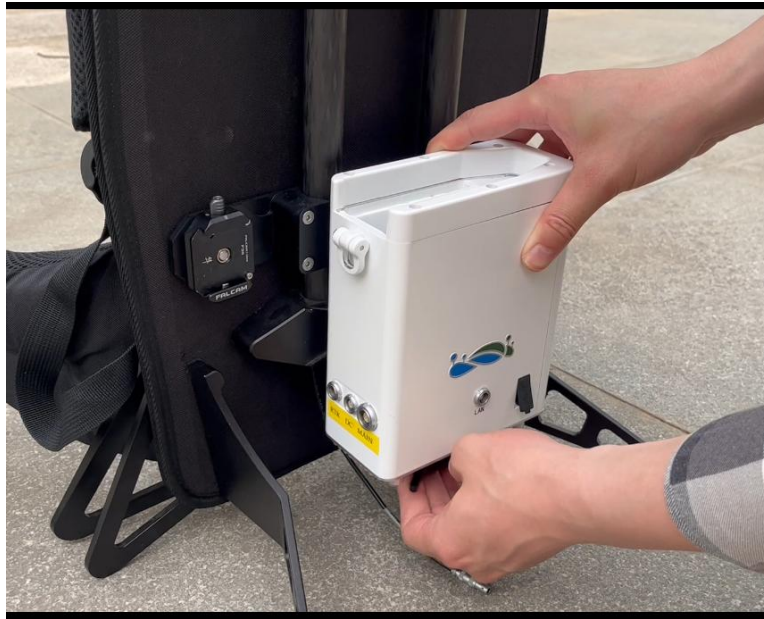
Figure 2-8 Aligning the battery compartment with the bottom screws and securing it
