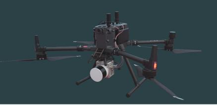
The LiAir X3C-H is a new compact high-performance UAV LiDAR system and is the upgraded version of the LiAir300 by GreenValley International. It adopts a new integrated design style and built-in high-resolution mapping camera, providing higher performance and convenient operation for power-line inspection, topographic surveying, agricultural and forest monitoring, and more.
