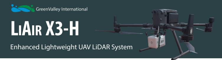
LiAir X3-H is the newest compact, high-performance unit in the LiAir series by GreenValley International. It adopts a new integrated design style and integrates lightweight LiDAR, self-developed inertial navigation, a high-resolution mapping camera and on-board computer systems providing new levels of efficiency.
